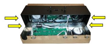
Route network cable through the top of device. Reattach the network cable coupler.
