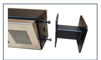
Run network cable (CAT5 or better) from POE+ switch or injector through bracket arm in direction shown, then attach bracket arm to load bearing ceiling supports using mounting hardware appropriate to the facility building materials. Note orientation of bracket arm to align viewing direction of clock in hallway or room.
