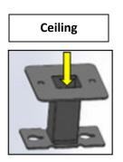
Remove the two screws and small cover plate, exposing the opening on the top of the device. Place the small cover plate over the opening on the side of the device, and fasten it with the two screws.
