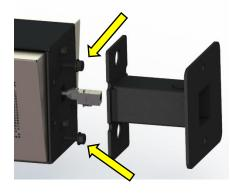
Pull ethernet cable from the wall through the bracket arm. Attach bracket arm to wall using mounting hardware appropriate to the facility building materials. Note keyhole orientation with narrow channel of keyhole at bottom.
